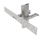
PIM-Guard® Antenna and RRU Cable Support Bracket with 22 ports for stackable hangers (up to 3 per port). Install with torque wrench set at 10 to 15 ft-lb to meet carrier PIM requirements.
