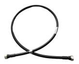
HELIAX® 1/2" Superflexible SureFlex® Jumper with interface types 7-16 DIN Male and 7-16 DIN Female, 3 m
