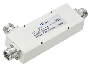
ValuDAS™, 20 dB, Air Directional Coupler, 578–3800 MHz, 4.3-10
