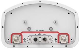
Kit with one 2-port sector antenna model LNX-6514DS-R1 (2x 698–896 MHz, 65° HPBW, 1x RET)
