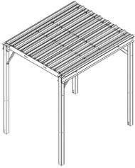
8'x12' Heavy Duty 18 gauge Protective Platform Canopy Kit (for MTC4038 platforms)
