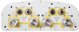
4-port sector antenna, 4x 1695–2690 MHz, 65° HPBW, 2x RET. Two pairs of AISG Input and Output ports to separately and independently control the RET on each array for operator sharing applications.
