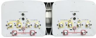
12-port sector antenna, 4x 698–960 and 8x 1710–2690 MHz, 65° HPBW, 6x RET with manual override. Bands cascaded SRET (Antenna 1 and Antenna 2).
