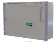
Heat Regenerated Dehydrator, 19 in rack mountable, 3.0 kPa (0.44 psig), with low pressure, high pressure, high humidity, power and system failure alarms, 110-240 VAC: 48V
