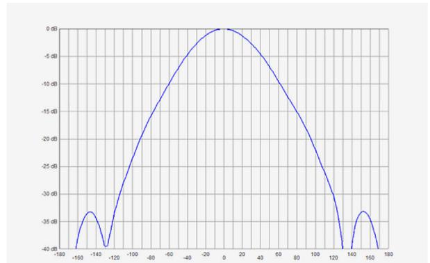
Typical 65° HPBW Pattern of a 4T4R MIMO Antenna
