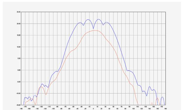
Comparison of a 65° pattern in Red vs Service Beam Envelope Pattern of an 8T8R Antenna in Blue (Service Beam shown with just 4 beam directions at  $\pm 10^\circ$  and  $\pm 30^\circ$ , as an example)
