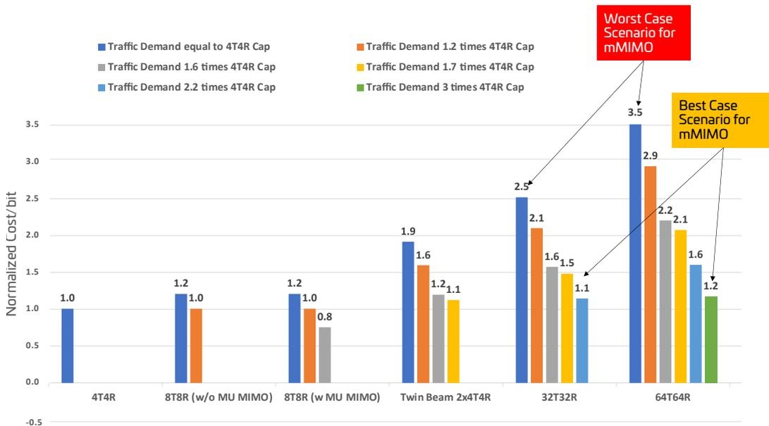
The chart below shows another way of representing the impact of traffic demand on the cost per bit of a configuration. The bar values below the normalized cost per bit line of 4T4R have a negative impact, while the bar values above the line have a positive impact—a lower cost per bit. It demonstrates that 8T8R with MU MIMO offers the best cost-per-bit ratio at the cost levels assumed across the configurations.
